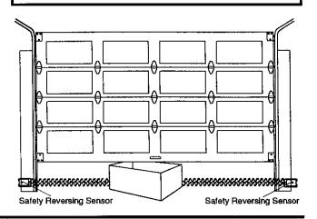
Failure to test and adjust the safety reverse system may result in serious injury or death to persons trapped by a closing garage door. Repeat this test once a month and adjust as needed.
